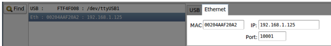
Figure 7.26: Ethernet connection details
